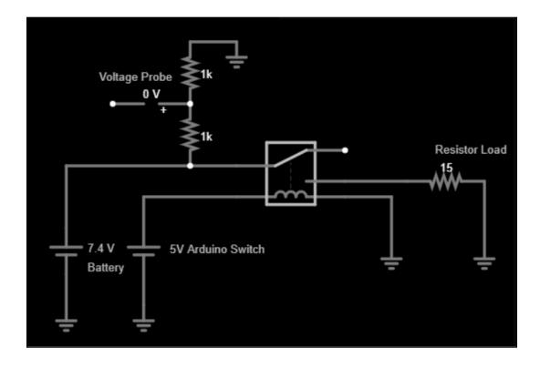
To protect the battery from overcharging and being damaged by the current from the solar panel, the team needed a protective overcharge circuit. Originally, the team planned to use a prefabricated charge control board but decided to design a circuit to better fit the project's specifications. The group designed and tested the circuit in LTSpice and then assembled the circuit physically on perf board.
