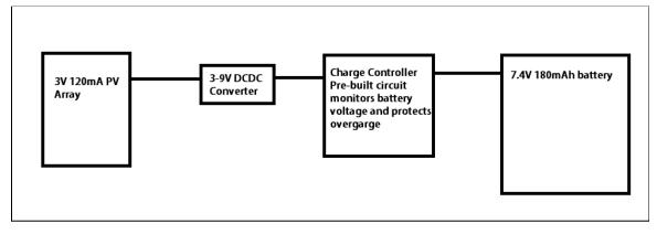
The initial design is a block diagram that helped guide the part selection and an idea of the physical construction of the project. Based on the client's requirements for charge time and battery capacity, there needed to be a minimum battery size of 100 mA and a solar cell that could charge the battery within 6 hours. Using a dc-dc converter to step up the PV voltage and a charge controller to protect the battery was achievable.
