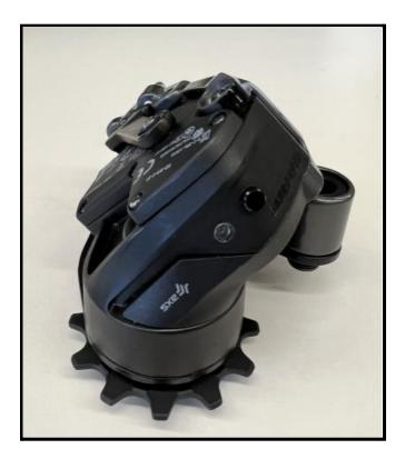
Once the derailleur is turned on, it is ready to be used on a ride as long as the battery is charged. If the battery is not charged, allow the solar cell to sit in the sun to charge before using the derailleur for a ride.
